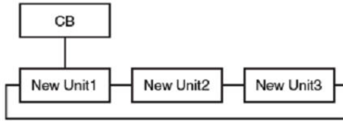
FIGURE 29 Case 1: Ring of potential PEs with one direct connection to the CB
